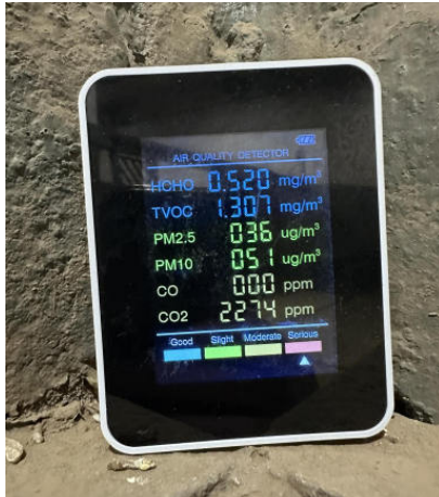
Picture 1. Air-quality monitor
